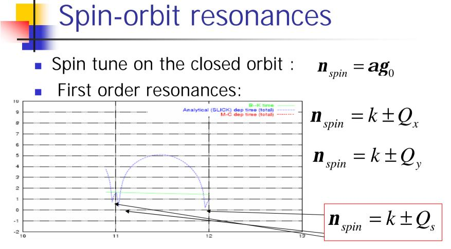
OCS ring depolarisation time with misalignments
