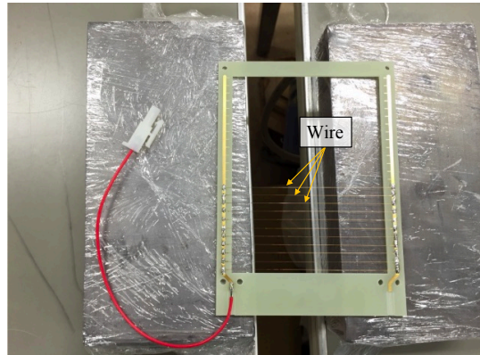
Figure 2.3: Photograph of two Si detectors. Figure 2.4: Electrostatic shield made of Cu-Be wires to protect the Si detectors.
