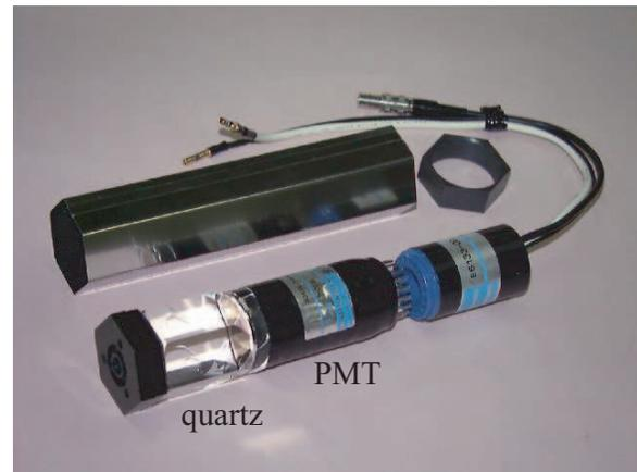
Figure 3.17: A pair of a quartz and a phototube used in the BBCs.
