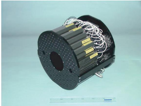
Figure 3.16: A picture of a BBC. It consists of 64 pairs of a quartz and a phototube.
