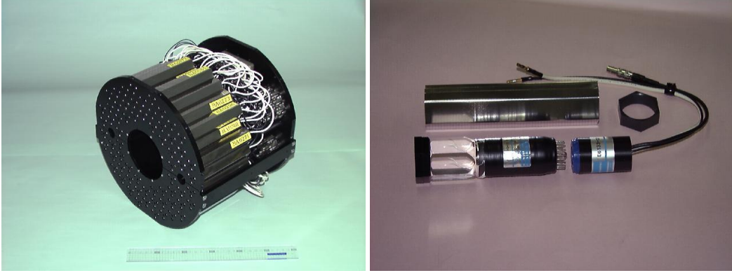
Figure 4.4: (Left) A picture of Beam-Beam counters module comprising 64 Čerenkov counters. (Right) A picture of quartz radiator and PMT.
