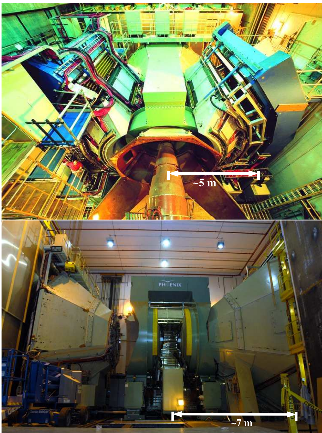
Figure 2.4: (Top) The photo of the PHENIX detector from beam view. Beams go up and down. The two spectrometers on the left and right side are the central arms. The blue detectors at the outermost are EMCal. The north muon arm was not installed at the time when the photo was taken. (Bottom) The side view of the PHENIX detector. Beams go left and right. The two spectrometers on the left and right are the muon arms. The structure labeled as PHENIX at the center is the magnet for the central arms. The east arm is moved in the bottom photo.
