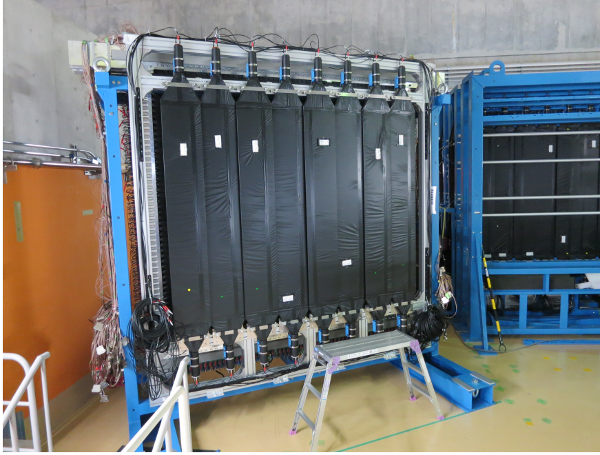
Figure 3.24: Photograph of the NeuLAND demonstrator with charged-particle veto counters.
