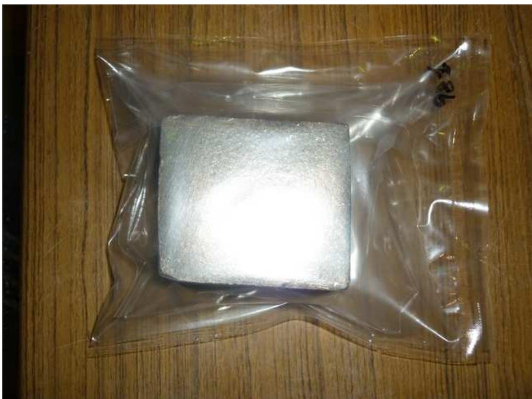
Figure 2.23: The Picture of  ${}^6\text{Li}$  target
