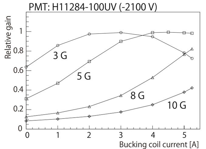
FIG. 8. Relative gains of an H11284-100UV PMT ( $-2100$  V) as a function of the bucking-coil current for  $B_y = 3, 5, 8$  and  $10$  G. The relative gain at  $B_y = 5$  G, which is larger than the maximum magnetic field at around PMTs of the water Čerenkov detector in S-2S, was able to be recovered up to  $\simeq 1$  by the  $20$ -turn bucking coil with the current of  $4.5$  A. The bucking coil was started winding  $30$  mm away from the PMT photocathode.
