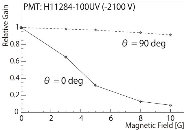
FIG. 7. Relative gains of H11284-100UV PMT at  $-2100$  V when the magnetic field of  $0, 3, 5, 8$  and  $10$  G was yielded in parallel ( $\theta = 0$  deg) and perpendicular ( $\theta = 90$  deg) to the PMT axis.
