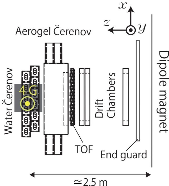
FIG. 2. A schematic drawing of the S-2S downstream particle detectors. The water Čerenkov detector is planned to be installed 2.5 m away from the S-2S dipole magnet, and the stray-magnetic field in parallel to the PMT axis ( $B_y$ ) was measured to be  $\leq 4$  G there.
