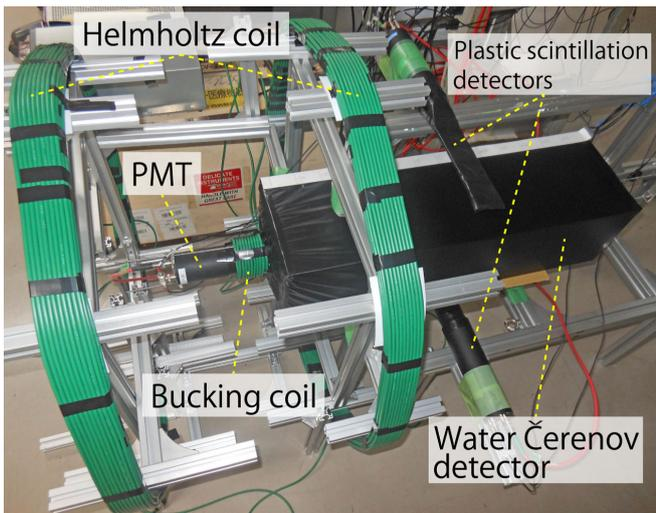
FIG. 4. A photograph of an experimental setup of the bucking-coil test.
