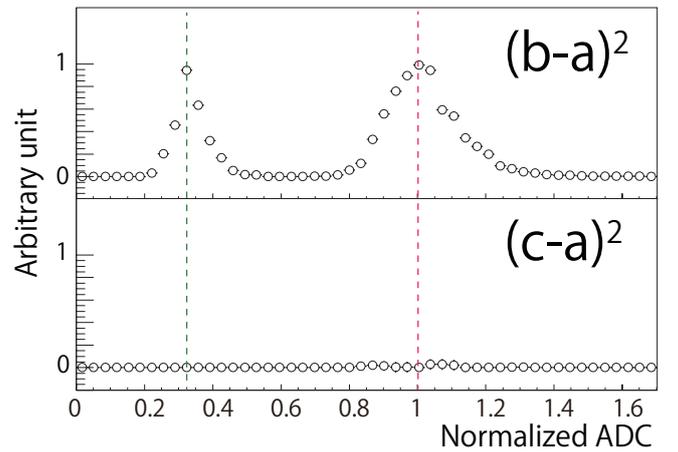
FIG. 10. Spectra of squares of residuals for (a)-(b) and (a)-(c). If two spectra is the exactly same, the square of residual becomes zero. An integrated charge by a signal of Čerenkov radiation was reduced by approximately 70% in the case of (b) as shown in a top panel  $(b-a)^2$ . On the other hand, the  $(c-a)^2$  spectrum distributes around zero, and it indicates the gain was able to be recovered by the bucking-coil implementation on PMT.
