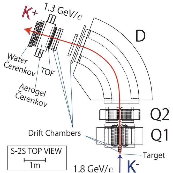
FIG. 1. A schematic drawing of S-2S top view. S-2S consists of two quadrupole (Q1, Q2) magnets, one dipole magnet (D), and particle detectors.  $K^+$ s with the momentum of 1.2–1.6 GeV/c are measured in S-2S.
