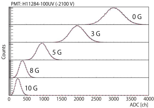
FIG. 6. ADC histograms of H11284-100UV PMT at the supplied high voltage of  $-2100$  V when the magnetic field of  $B_y = 0, 3, 5, 8$  and  $10$  G was yielded.
