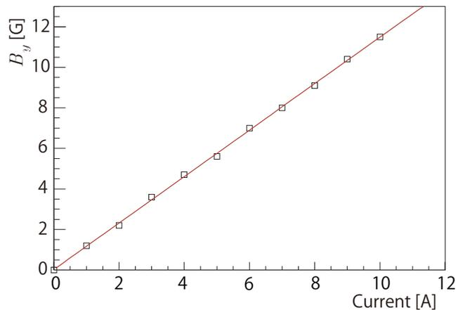
FIG. 5. A measured relation between the current and  $B_y$  at the center position of the Helmholtz coil we constructed.
