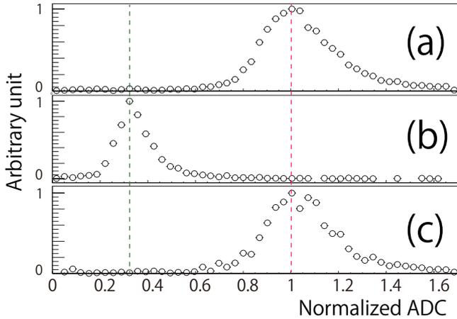
FIG. 9. Normalized ADC spectra in the cases of (a)  $(B_y, I_B) = (0 \text{ G}, 0 \text{ A})$ , (b)  $(B_y, I_B) = (5 \text{ G}, 0 \text{ A})$ , and (c)  $(B_y, I_B) = (5 \text{ G}, 4.5 \text{ A})$ .
