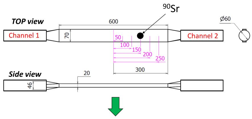
Measured the time difference between signals from two PMTs.
