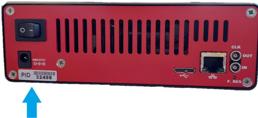
Fig. 4.1: PID location taking a CAEN desktop unit as an example (the number in the picture and the device model are purely indicative)
